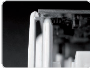
Board lock too tough.
