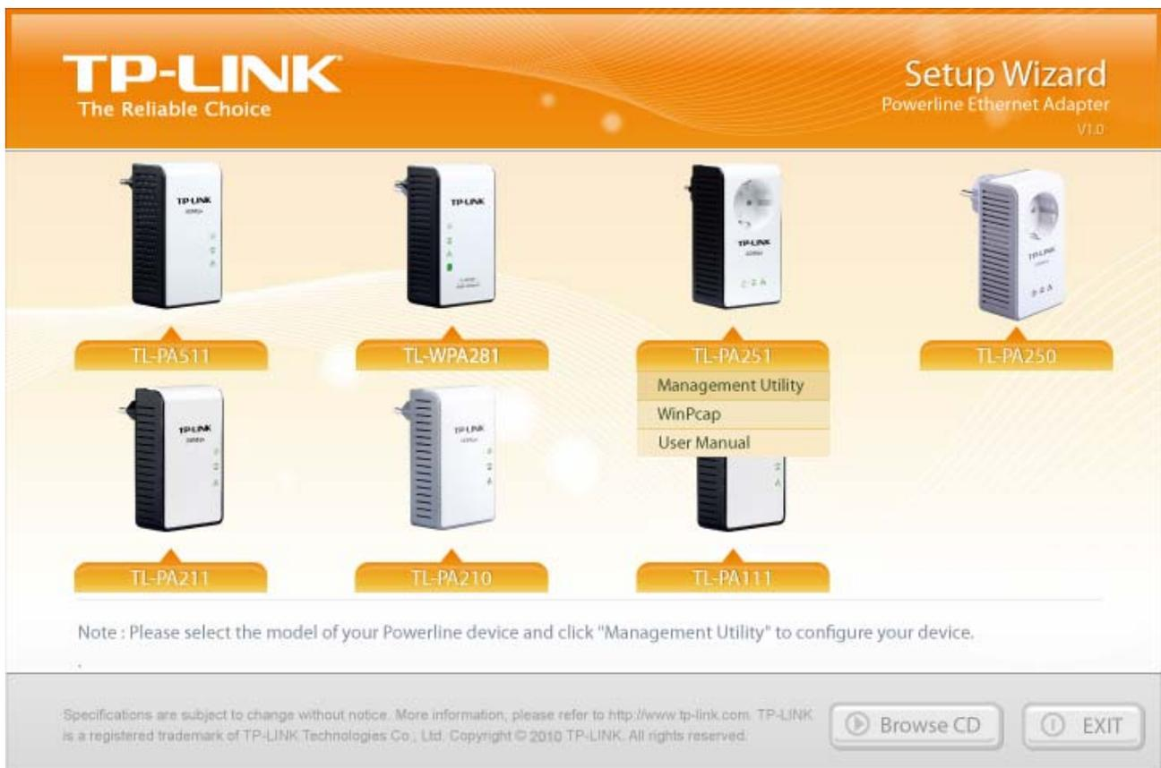
Step 2: Select **TL-PA251** and click **Management Utility** and the program installation process will carry out and copy all the necessary files to your system. Follow the instruction step by step to finish the installation.
