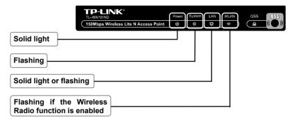
Note If the LEDs display abnormally, please check to see if all the cable connectors (power adapter and Ethernet cable) are well connected to your device
