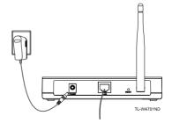
Note If the distance between the outlet and the Access Point is too long to supply the power, you can refer to the Power over Ethernet(PoE) solution in Appendix B: With PoE Setup.
