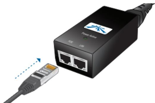
2. Connect an Ethernet cable from your LAN to the Ethernet port labeled **LAN** on the *PoE Adapter*.
