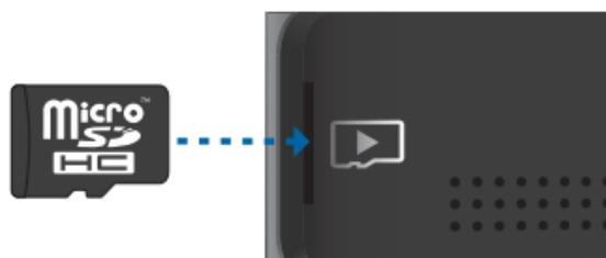
To remove the microSD card, push the card in to release the lock. Pull the card out.
