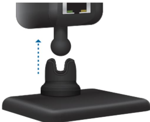
4. Attach the *airCam Mini* to the *Wall Mount Bracket*.
