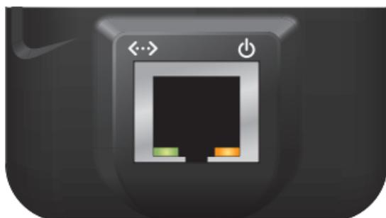
↔ **Ethernet** The Ethernet LED will light steady green when an active Ethernet connection is made and flash when there is activity.
