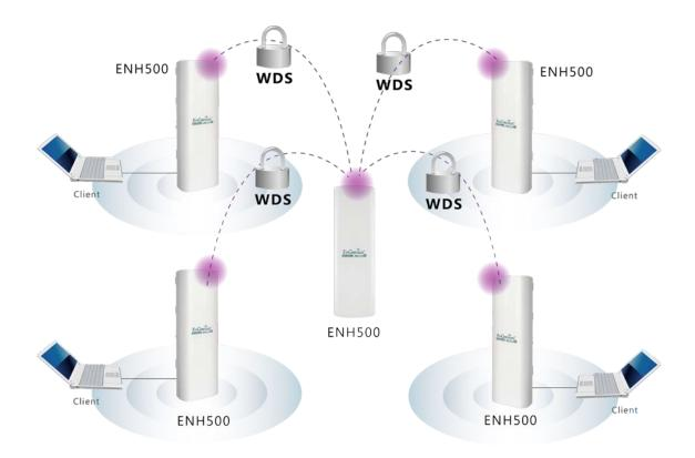
WDS Bridge Mode is unlike Access Point. APs linked by WDS are using the same frequency channel, more APs connected together may lower throughput. Please be aware to avoid loop connection diagram, otherwise enable Spanning Tree Function.
