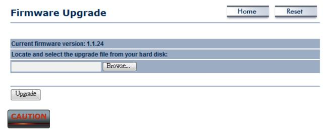
Upgrade process may take few minutes, please do not power off the device and it may cause the device crashed or unusable. ENH500 will restart automatically once the upgrade is completed.
