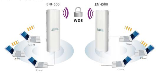
Not every Access Point device has support WDS in Access Point Mode. It is recommended using ENH500 if you would like to use this service.
