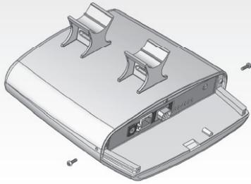
**STEP 10** The StationBox™ is completed now and you can close it with Removable cover (before placing the Removable cover you can connect appropriate cables to your PCB).
