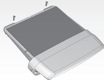
**STEP 8** Whole entity fix by using 2 screws according to the picture.
