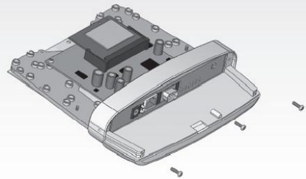
**STEP 7** Attach antenna using 2 screws at the upper part of antenna (using free holes), according to the picture. Then, connect the pigtail to the radio.
