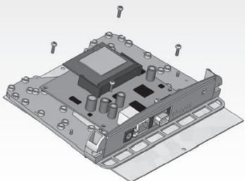
**STEP 5** Insert Lower part into "Base" according to the picture.
