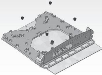
**STEP 3** Place the board of your device into holes on the front side of part "Base" and on appropriate positions considering the Spacers.
