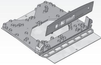
**STEP 2** Insert Spacers into appropriate holes on the part "Base". Amount of Spacers and its location depend on the type of board you want to install.
