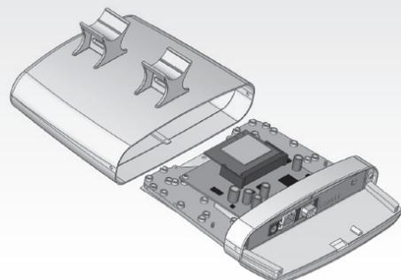
**STEP 9** Whole entity fix by using 2 screws according to the picture.
