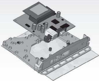
**STEP 4** Screw the board of your device by using applied screws. Amount of the screws depends on amount of the Spacers that are used for your board.
