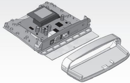
**STEP 6** Fix the Lower part by using 3 applied screws.
