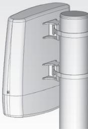
The StationBox™ can be installed on the mass or console by using applied Cable ties.
