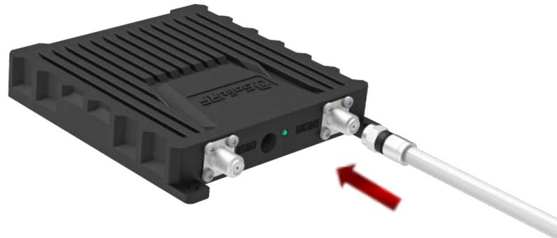
3. Connect the indoor antenna to the "INSIDE" port on the booster.
