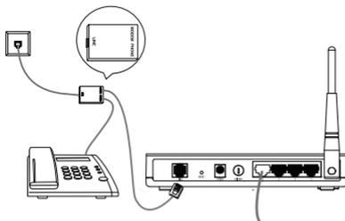
**Note** If no telephone is needed, please connect the LINE port of the Modem Router to the wall jack using the telephone line directly.
