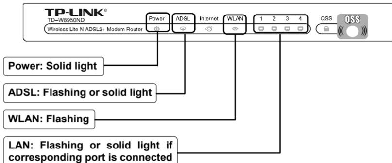
**Note** If the LEDs display abnormally, please check to see if all the cable connectors (power adapter, phone line and Ethernet cable) are well connected to your device. With the phone line well connected, if the ADSL LED turns off after flashing, please contact your ISP to ensure that your internet connection is active.
