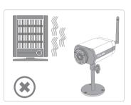
• Do not place the camera near devices that emit radio waves, such as mobile phones
