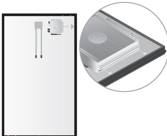
3. Secure the *Microinverter* to the inside edge of the *Solar Panel* using the two included mounting bolts. Ensure that the neighboring edge of the *Microinverter* is still attached to the corner frame edge before inserting the mounting bolts.
