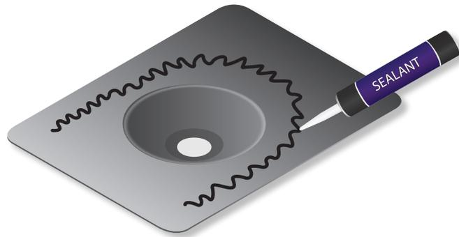
14. Slip the *Flashing* into place underneath the upper course of shingles and lower it in to place over the roof mount. The flashing should be installed with the Ubiquiti logo towards the front.
