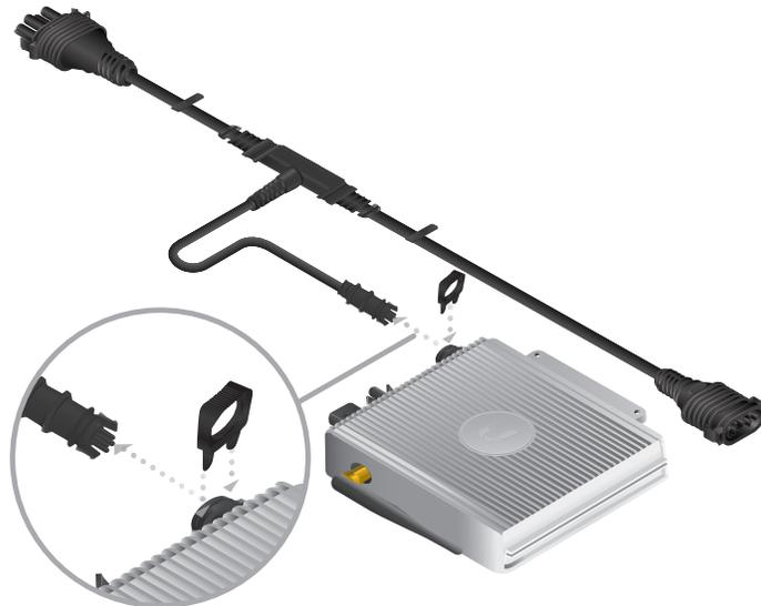
3. Connect the AC trunk cable (that was previously connected to the Microinverter) to the *Output* connector on the Solar Gateway.
