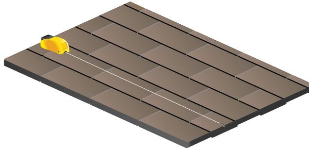
2. Mark the location of the second row of roof mounts by placing a parallel chalk line above the first, using the following guidelines:
