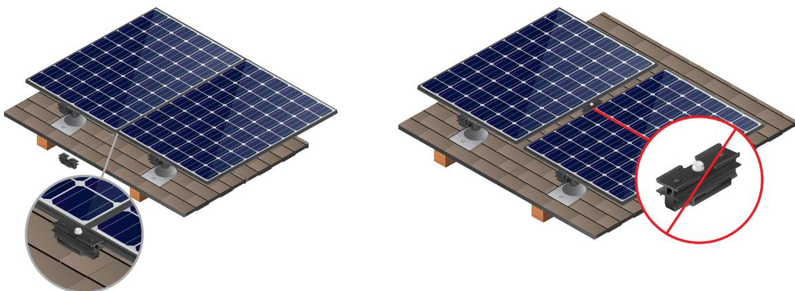
When you have multiple mounts on a *Solar Panel* or one right next to a connector, do not install the mount closest to the connector. Leave it loose temporarily, allowing the *Solar Panel* to drop quite a bit where they come together and make it easier to level the array panels.
