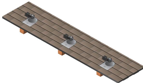
7. Secure and tighten each mounting assembly bolt (19 N-m torque) and remove the leveling string before installing the trim cover.
