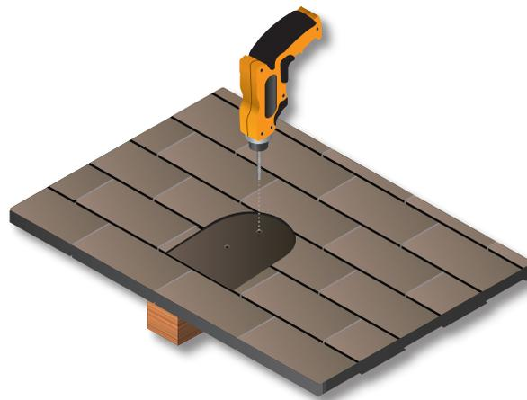
10. Cover both hole openings with roofing sealant. This will ensure watertight installation once the lag screws have secured the roof mount to the rafter.
