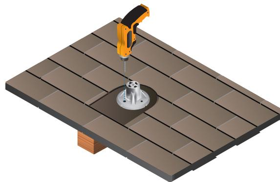
9. Remove the roof mount temporarily and finish predrilling two 3/16" (4.8 mm) holes approximately 2" (50 mm) deep.
