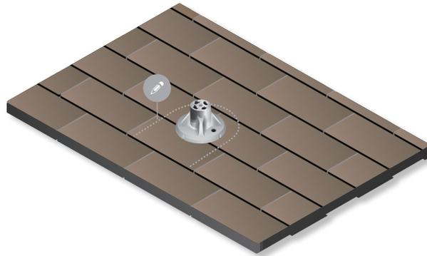
8. Once the shingles have been trimmed, position the roof mount over the rafter center and start predrilling the two holes that will be used to secure the roof mount to the rafter. Use the shingle cutout and the two smaller holes on the roof mount as a guide for positioning. (Note: To avoid damaging the roof mount, do not drill the holes completely through with the roof mount in place.)
