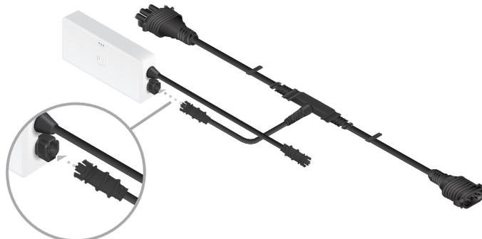
4. Connect the *Input* cable on the Solar Gateway to the four-prong connector on the Microinverter.
